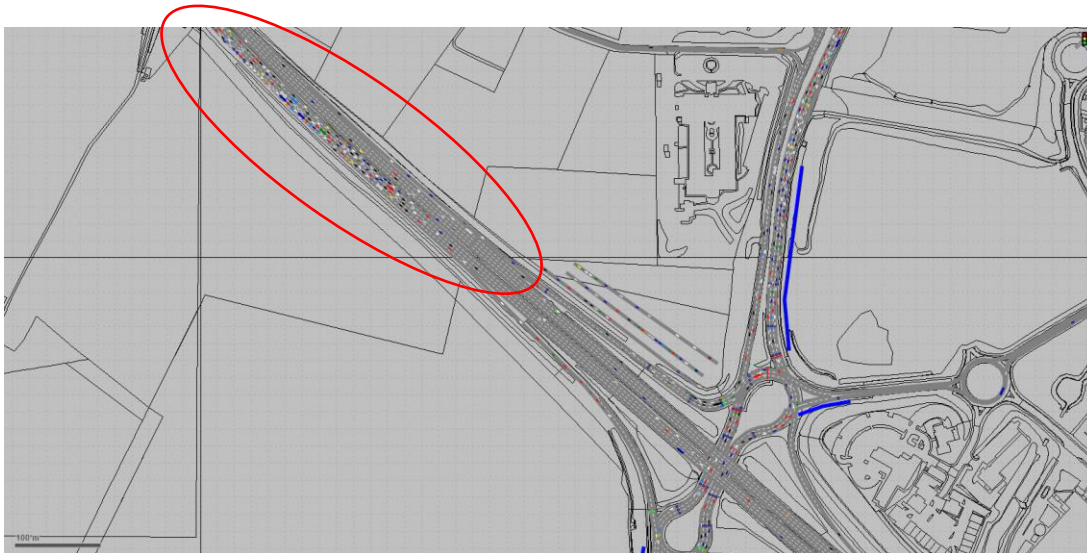
M1 J15a – Extent of queues from M1 / A43 roundabout causing disruption on M1, which has almost reached M1 J15.
