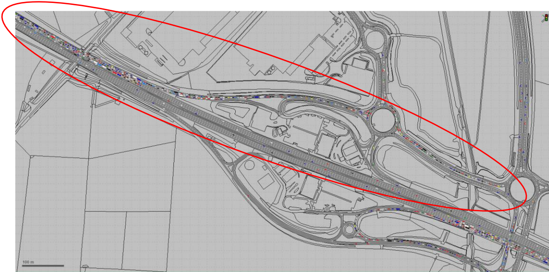
M1 J15a – Queues from A43 / Swan Valley and A43 / A5123 affecting M1
